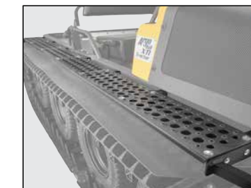
Catwalk - 6.25" (160 mm) steel platform along the length of the vehicle. Includes a 10" (255 mm) mud flap.
