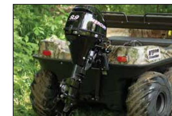
Outboard motor bracket - Accepts an outboard motor of up to 9.9 HP.
