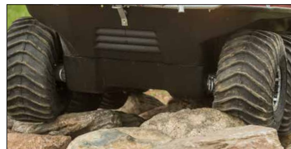
A full-length skid plate protects the underbody from damaging brush and rocks, and allows the Scout to resist hanging up on trail obstacles.
