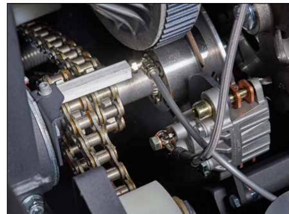
Auto Chain Lubrication Simplifies routine maintenance to ensure smooth, dependable operation for frequent users.
