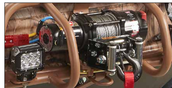
The powerful Warn winch , standard on Scout models, provides up to 3,500 lb. (1,588 kg) of pull for vehicle recovery or heavy loading.
