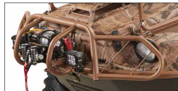
A robust brushguard mounted up front fends off impacts from brush and branches.
