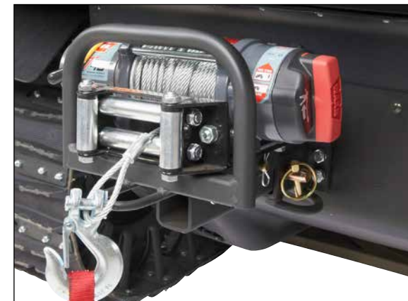
Rear Receiver Winch Mount This rear receiver winch mount and wiring harness allows rear mounting of the standard Warn winch to get more use out of its heavy pulling and loading capability.
