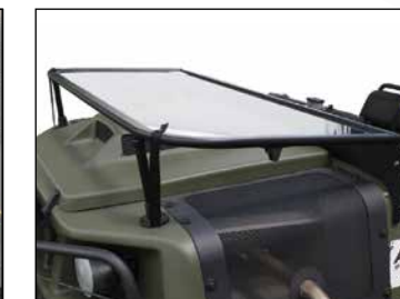
Windshield - Scratch-resistant acrylic in an aluminum frame, features fold over hinge for storage and a mounting location for the optional windshield wiper accessory.
