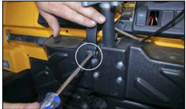
Figure 3-3. Adjustment on cam lever.
