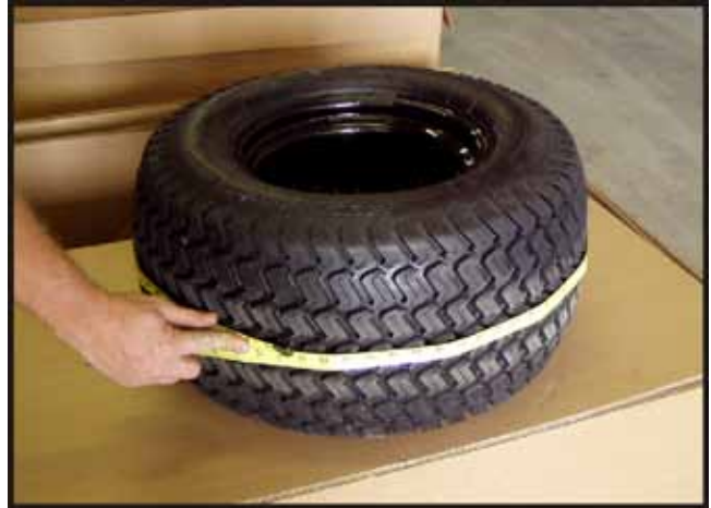
Figure 11-1. Measuring the tire.
