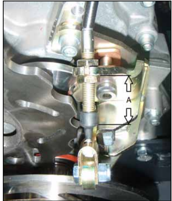
Figure 7-14. Adjusting the parking brake - disc brake.
