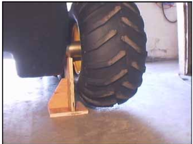
Figure 9-1. Correct placement of blocks
