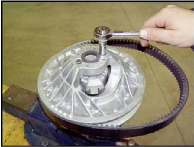
Figure 7-2a. Loosen jam nuts.
