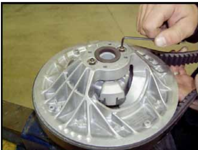
Figure 7-2b. Turn the adjustment set screw.
