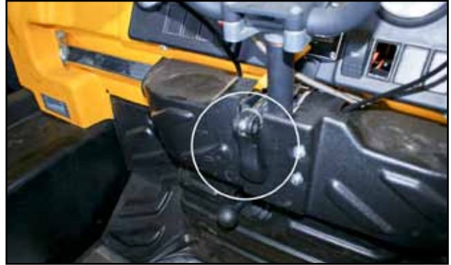
Figure 3-2. Steering position adjustment.
