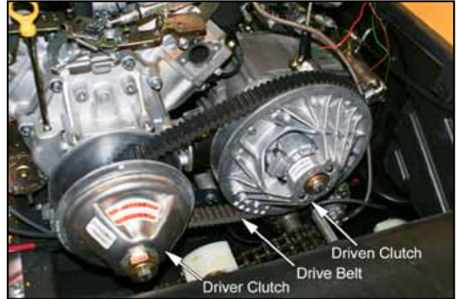
Figure 7-2. Location of drive clutches and drive belt.
