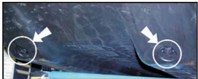
Figure 5-1. Location of rear drain plugs.
