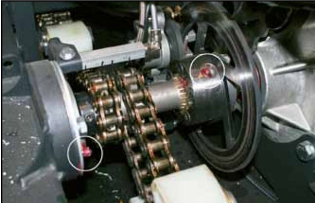
Figure 6-6. Output shaft grease fitting.
