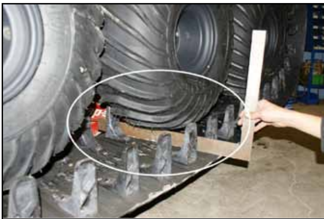
Figure 11-12. Measuring the gap of the mid tires.
