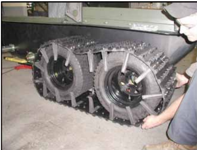
Figure 11-3. Positioning on wheel hubs.
