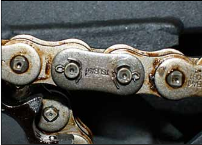
Figure 7-5. Chain connection link components.
