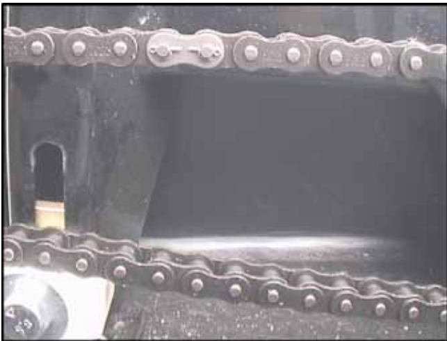
Figure 7-6. Installing the connecting link.
