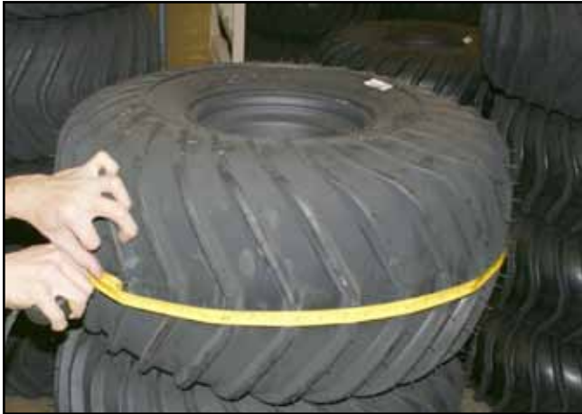
Figure 11-7. Measuring the tire.
