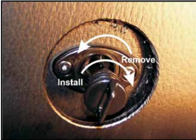
Figure 5-2. Removing and Installing the drain plug.
