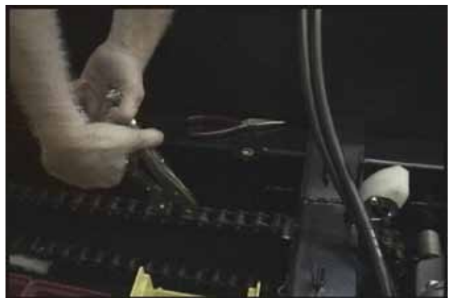
Figure 7-4. Holding chain together to insert connecting link
