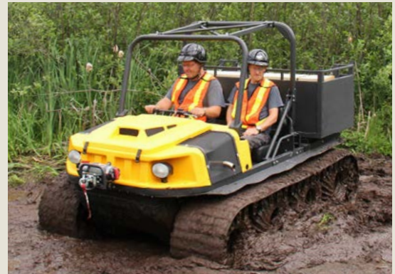
The low center of gravity and full-time, eight-wheel drive provides sure-footed traction and maneuverability.
