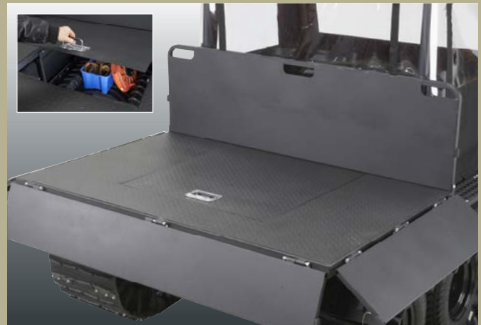
Optional, easily removable flatbed platform with access panel to storage area. Custom cargo configurations can be created by adding stakes, hinged or fixed side panels and tailgate.
