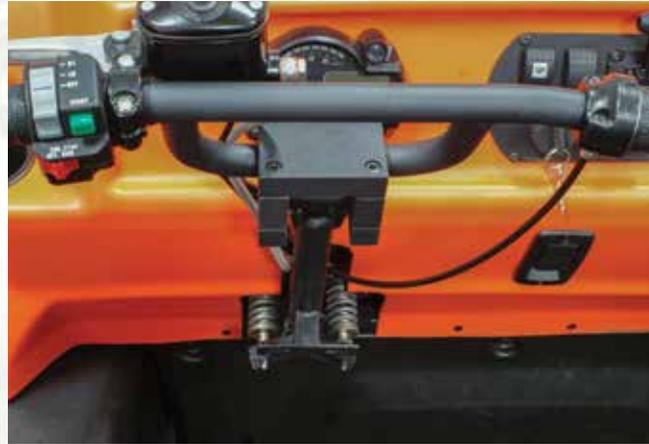
handlebars and the brake system. APS delivers a progressive, dual rate steering system that results in easier, smoother turning motion – plus a four-time wider range of steering motion – for greater driving confidence and improved steering.
