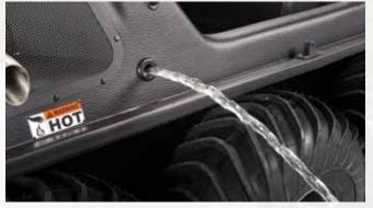
**Bilge Pump** A built-in bilge pump quickly and effectively evacuates water that enters an ARGO XTV.
