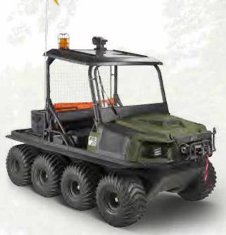
The Conquest Pro 800 XT-L 8x8 is equipped for emergency response with a ROPS protection cage with roof, a front windshield with wiper, plus a stretcher, vice, spotlight and flashing light. It's available in Industrial Yellow or Green.
