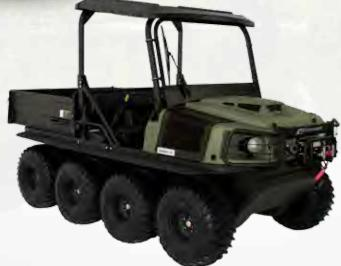
The Conquest Pro 800 XT-X 8x8 offers a ROPS protection cage with roof, a front windshield with wiper, and a power rear dump box. It's available in Industrial Yellow or Green.
