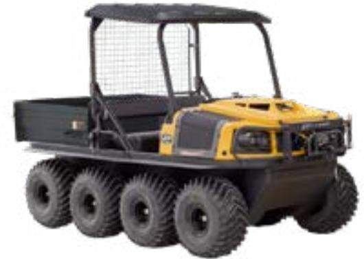
The Conquest Pro XT-X 8x8 comes standard with a ROPS protection cage with roof, rear mesh and a power rear dump box. It's available in Industrial Yellow or Green.
