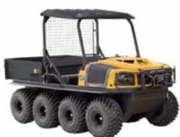
The Conquest Pro XT-X 8x8 comes standard with a ROPS protection cage with roof, rear mesh and a power rear dump box. It's available in Industrial Yellow or Green.
