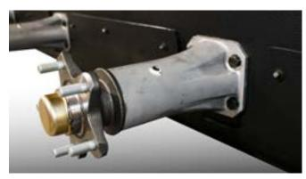
Heavy Duty Axle Heavy duty 1.5" forged axles in oil bathed reinforced housings.
