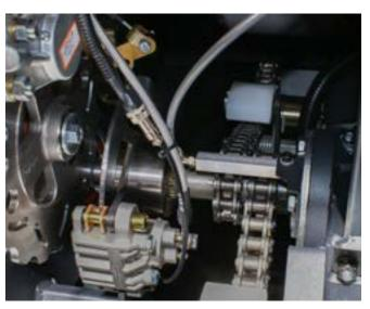
Auto Chain Lubrication Simplifies routine maintenance to ensure smooth, dependable operation for frequent users.
