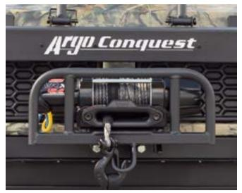
4500-Pound WARN Winch Conquest come equipped with a mighty 4500-LB WARN Winch for the ultimate in utility, ease-of-use and durability. The winch is conveniently operated via an on-dash actuator.
