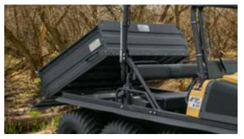
Power Dump Box The XT-X solid steel Power Dump Box can move bulk loads up to 1,000 lbs (450 kg).
