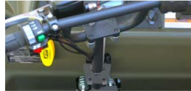
system. APS delivers a progressive, dual rate steering system that results in easier, smoother turning motion for greater driving confidence and improved steering.
