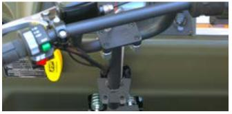
system. APS delivers a progressive, dual rate steering system that results in easier, smoother turning motion for greater driving confidence and improved steering.
