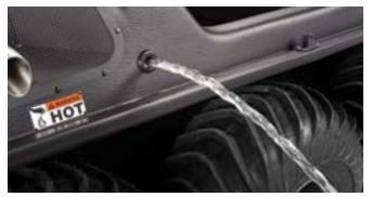
Bilge Pump A built-in bilge pump quickly and effectively evacuates water that enters an ARGO XTV.
