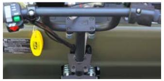
ARGO Progressive Steering (APS) ARGO Progressive Steering (APS) is an innovative steering technology used on our XTVs. Used in conjunction with the Classic transmission, APS adds a spring element between the handlebars and the brake
