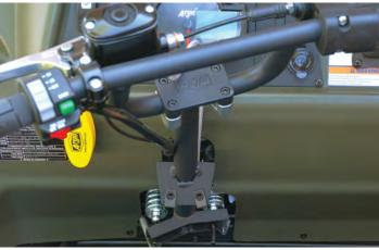
Steering is now effortless, with an increase of a 4-times-wider range of steering motion that offers the smoothest turning available in an ARGO XTV.
