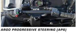
Operated in conjunction with the Admiral transmission, APS adds a spring element between the handlebars and the brake system to deliver a progressive, dual-rate steering system which results in an easier, smoother turning motion that instills driver confidence while offering improved steering.
