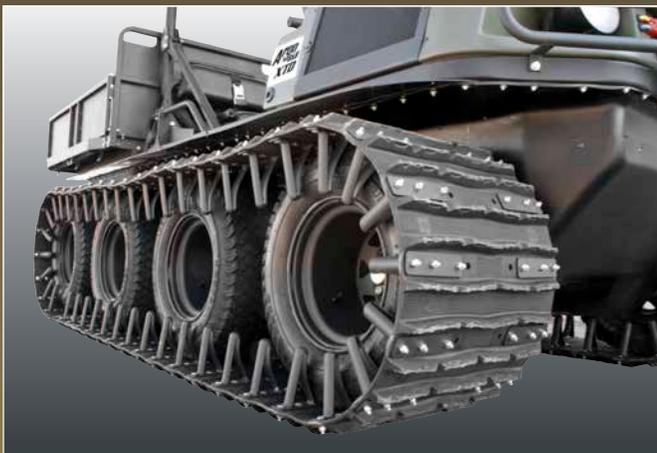
Optional 18" (457 mm) rubber tracks with heavy duty steel guides on high impact resistant 24" (610 mm) turf tires and reinforced rims.
